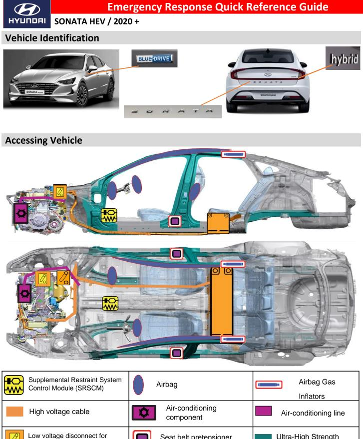
Low voltage disconnect for high voltage
